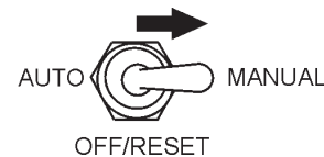
Figure 40. MPEC Control Switch (Manual Position)
